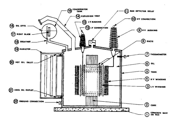
Figure 2: Cross Section of a Power Transformer
