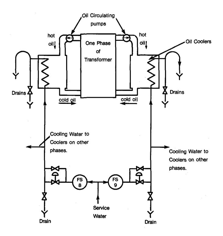
Figure 5: Cooling System for Main Transformers at Bruce "A" NGS.
