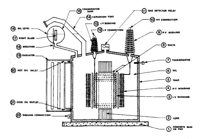
Figure 3: Cross Section of a Power Transformer
