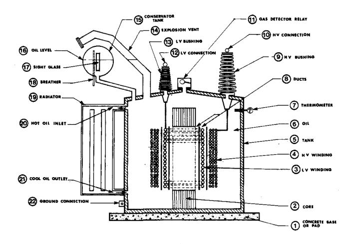
Figure 4: Cross Section of a Power Transformer
