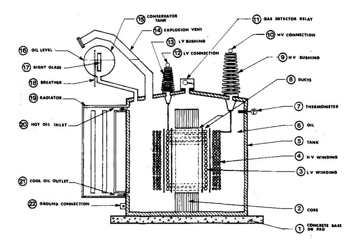
Figure 1: Cross Section of a Power Transformer
